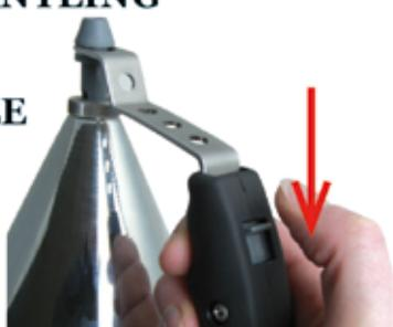
1. Press the locking button down to unlock the bar and the nozzle.
