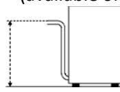
**IN THIS CASE, THE DRAIN CONNECTION MAY BE NO HIGHER THAN 1 M. ALWAYS CHECK THAT THE DRAIN WORKS PROPERLY AND IS NOT BLOCKED.**
