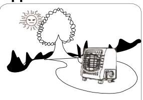
Do not place the heater in direct sunlight, find a Shady location, away from sand and soil ground.
