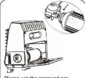
Please use the approved gas Cartridge and fit it in the way shown in the figure on the heater. 3
