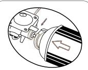
The gas cartridge groove must Be fitted as the above picture illustrated in order to match the guide on the gas regulator.
