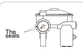
Check that the seals (between the appliance and the Gas container) are in place and in good condition before connecting to the gas container Do not use the appliance if it has damaged or worn seals
