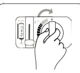
Turn the Control Knob to the "O" position to switch off the gas supply.
