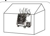
The heater must be situated in a Well-ventilated place or room when the gas heater operates because oxygen will be consumed.
