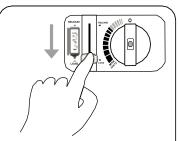
Make sure that the Control Knob is At the "O" position. Press the Cartridge Level button to the "LOAD" position.
