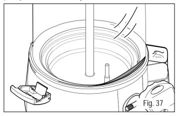
Fix the bowl to the machine body using the relevant hook-on handles, as illustrated in the figure;
