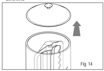
slide the mixer upwards to remove it, keeping it in line with the central rod until the bottom slot of the mixer itself is level with the rotation pin;
