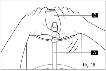
slide the mixing auger upwards with one hand, taking care to grip it by the rotation pin:
