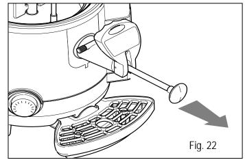
press the button (A) securing the tap to the machine and then remove the tap (B) with both hands, as illustrated in the figure;
