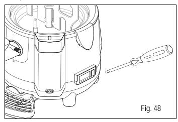
remove the used battery and fit a new one in its place, taking care to comply with the polarities indicated;
