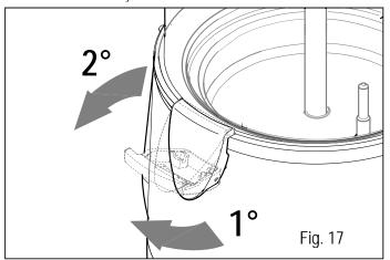
release the bowl from the machine body, using two fingers to prise it away
