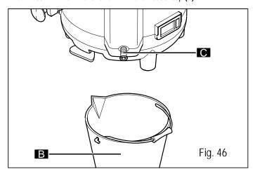
pull out the cap (C) with a firm movement and wait for all the water to empty out from the boiler tank.
