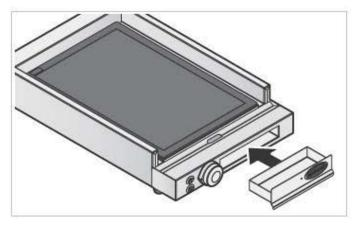
Before using the fry-top for the first time, insert the fat-collection drawer supplied in the front, as shown in the figure.
