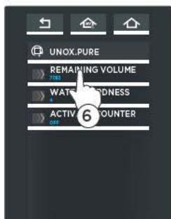
Select the "remaining volume": the residual litre count until the filter needs to be replaced appears on the display.
