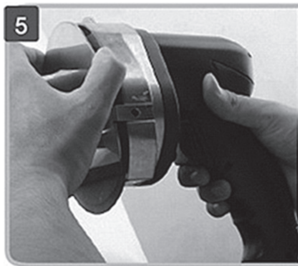
Attach the knife protector and Lock screw
