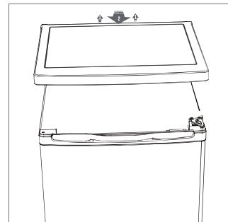
3. Unscrew top hinge and then remove door and place it on a soft pad to avoid scratch.
